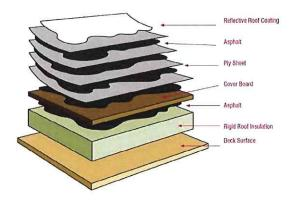
TPO Roofing – Quicker, cheaper & easier to install, offers rebates & significant energy savings. Must install catwalks to avoid puncture. If there is damage, it is easy to locate and patch. Can lay 4" of insulation to achieve high R value insulation rating.
